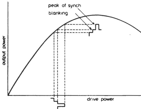
Fig. 4 Klystron transfer characteristic
