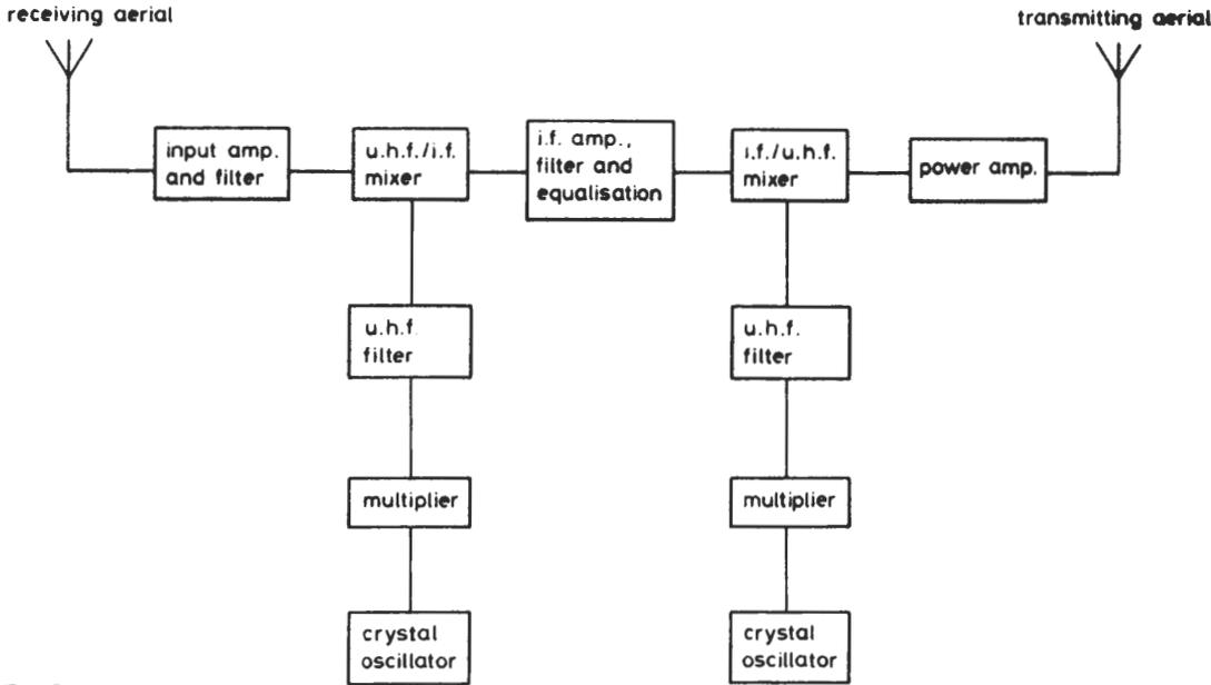
Fig. 2 Block diagram of typical transposer
