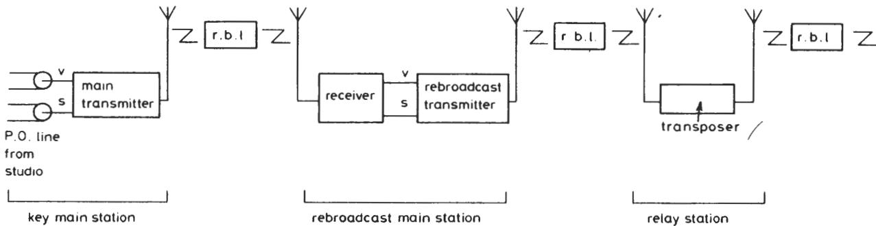
Fig. 3 Typical transmission chain
