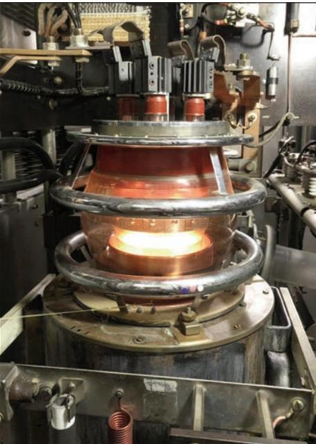
A BY1144L triode valve in the LH modulator position in a MWT BD272 transmitter (Neale Bateman)
