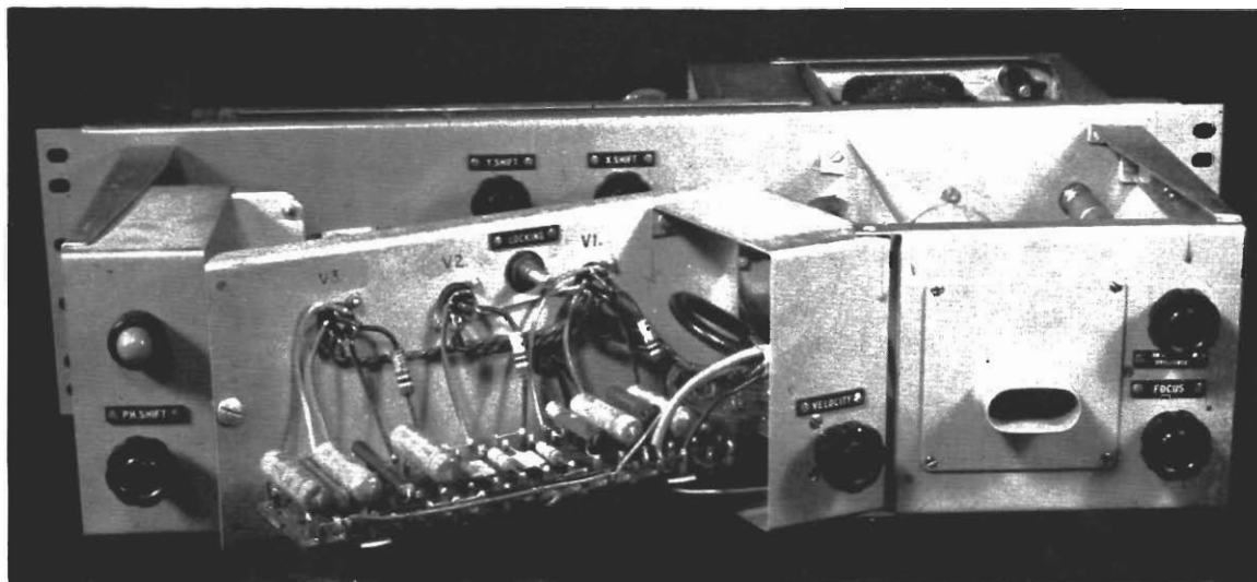
PLATE VIII. Frequency-checking Monitor Type FCM: Front View with Cover removed and Hinged Sub-panel swung forward
