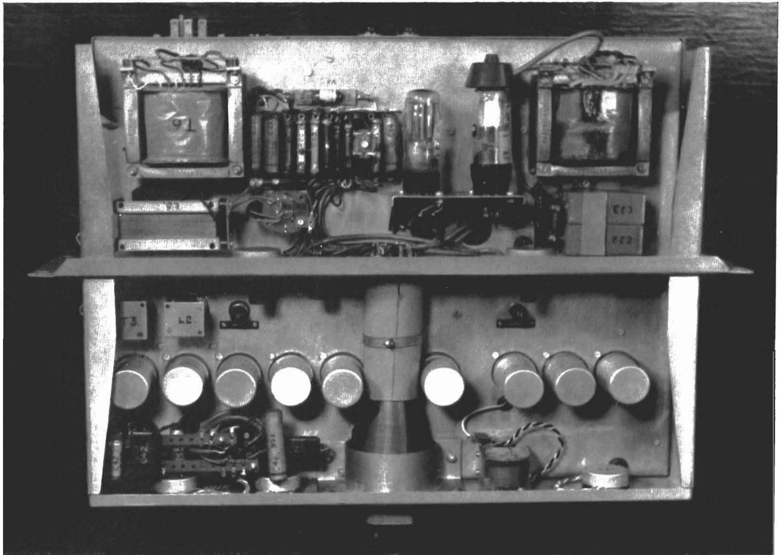
PLATE VI. Frequency Comparator Type FRC.2BM: Plan View with Covers removed
