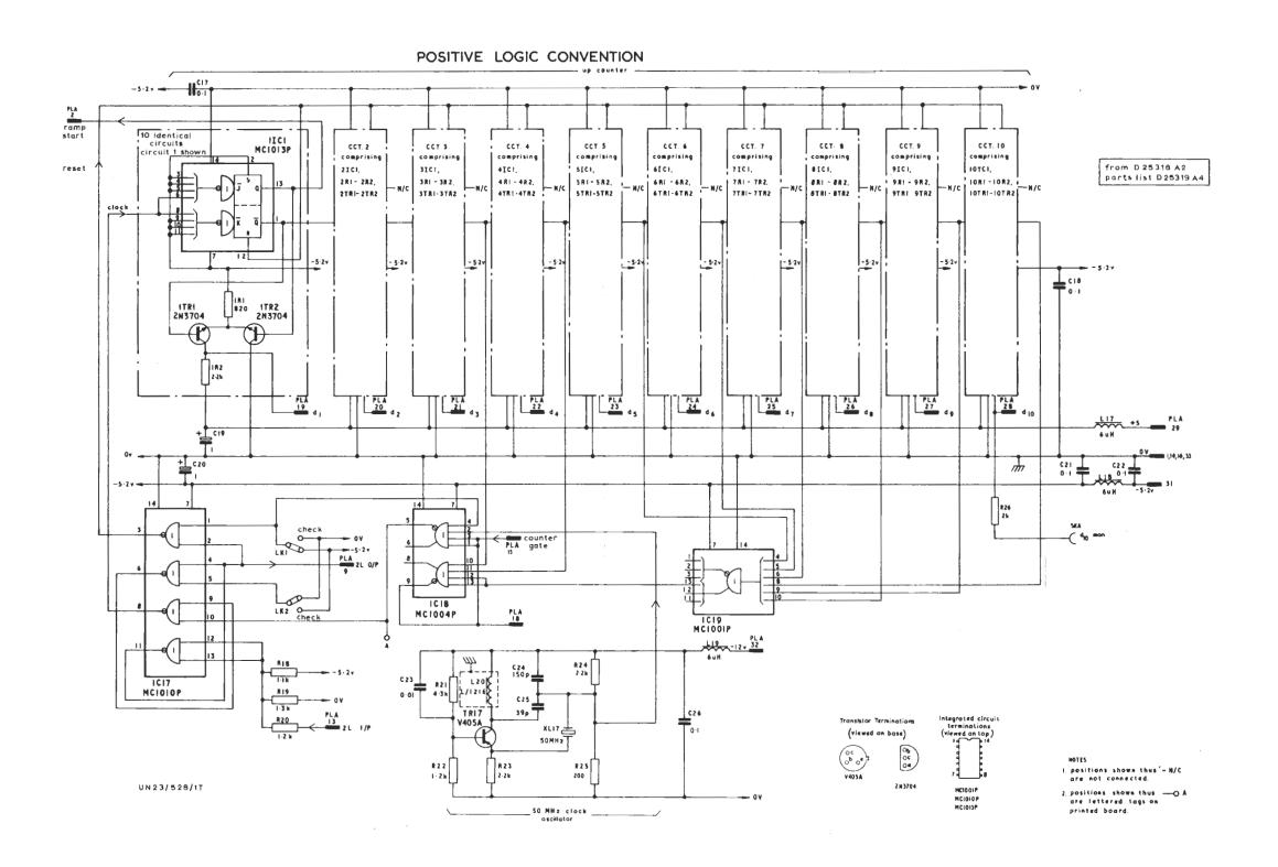
Fig.2 Circuit of the Counter and Clock Unit UN23/528
