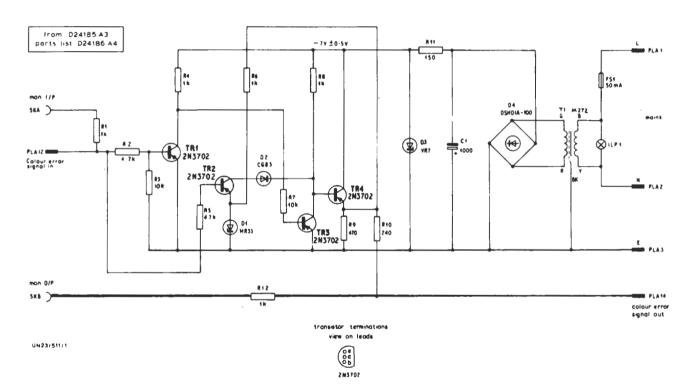
Fig. 1. Circuit of the Error Inverter UN23/511
