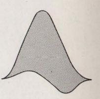
MIXED DISTORTIONS In this 10-T pulse the distortion comprises a mixture of the previous three examples,
