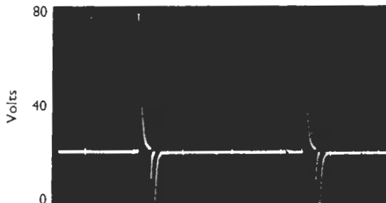
Waveform 3: V1A, Pin 6 Apply two volts of line-sync pulse to the Sync
