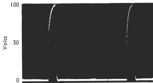
Waveform 2: V2, Pin 1 (Tag 5) Amplitude of pulse, 100 volts.
