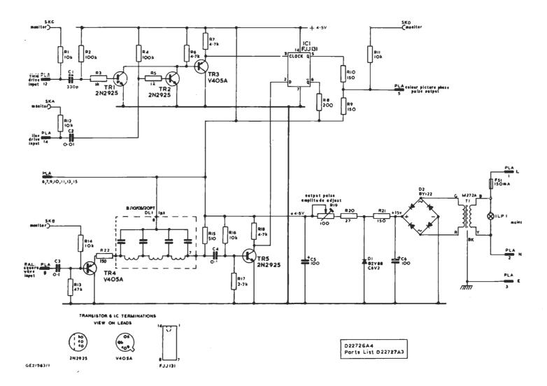
J=ig. Circuit of the Colour-picture Phase Pulse Generator GE2/563
