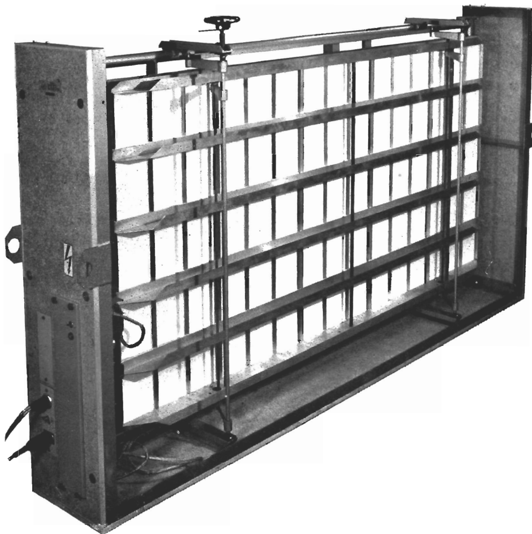
Fig. 1.2. Rear View of EMT 140 with Case Removed Showing Damping Plate
