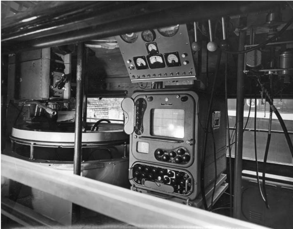
Interior view showing camera control position and camera lift in down position. Aerial turning mechanism is also visible.
