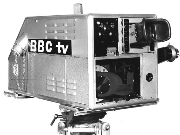
Showing optical folding and filter wheel assembly
