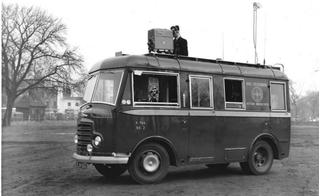
Roving Eye II ready to rove. Camera operator in place and steerable aerial to the rear.
