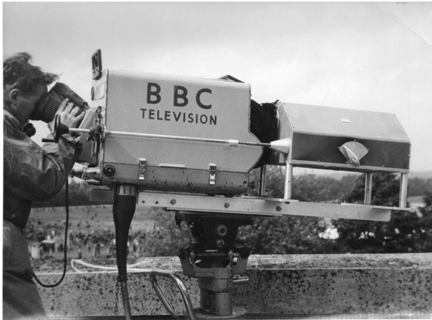
Photo of prototype Zoom lens fitted to one of the cameras used to televise the racing at Royal Ascot 12 June 1951 (BBC Photo)
