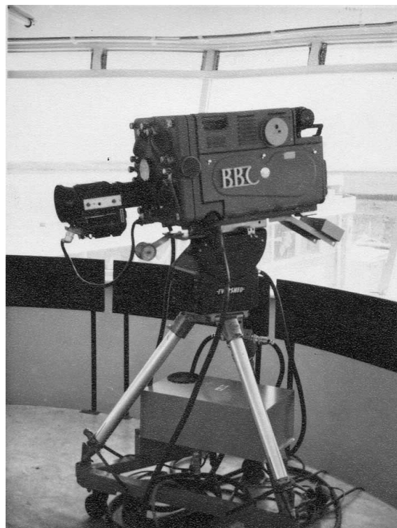
Photo of a later zoom lens on a Marconi Emitron Mk III from about 1953 (no date on photo but the Evershed name is visible).
