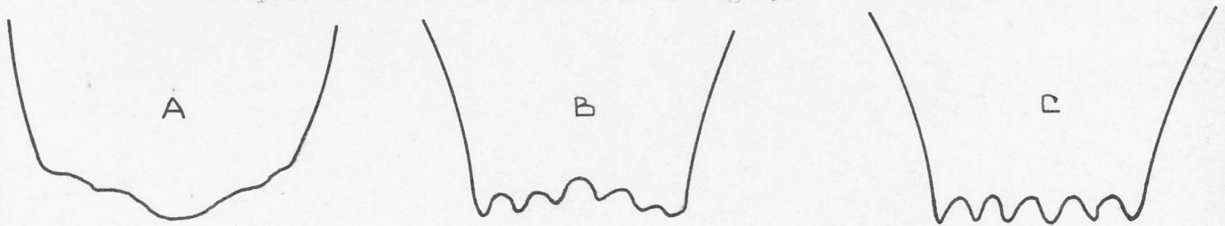
Fig. 3. TYPICAL RETURN LOSS RESPONSES
