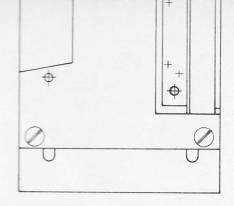
THROUGH HOLE PLATED BOARD, ALL LEADS PASSING THROUGH BOARD NOT TO BE BENT AFTER ASSEMBLY
