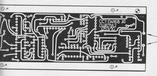
TO BS4584,+CL5.2, EP-GC-Cu-3, 6±O.2O (EPOXIDE WOVEN GLASS CLAD ON BOTH SIDES Jum THK. COPPER)
