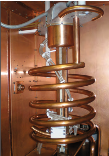
RIZ OR250K sender, second output coil showing motorised, water-cooled coil tap (Dave Porter)
