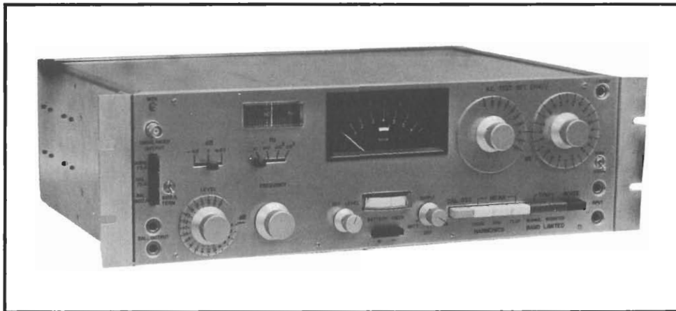
AC TEST SET. Within the one housing are contained a tone source, amplifier detector, test-programme meter and noise meter. As shown, the test set is for mounting on 19-inch bay; for portable operation, a carrying-case incorporating a battery-pack is used.
