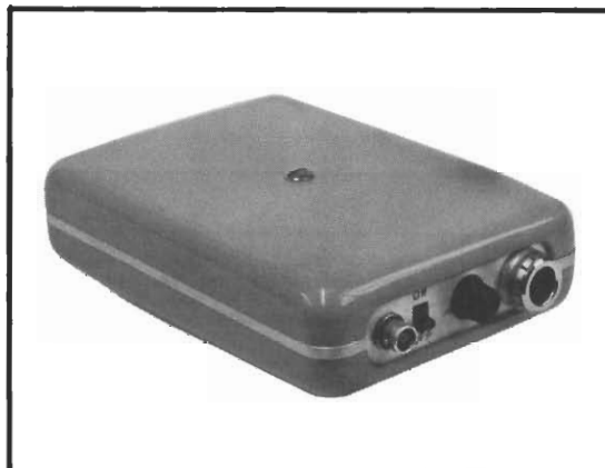
VHF RADIO MICROPHONE. This new, compact device has an output power of 250mW in the range 45-65MHz. An FET RF power output stage is used for stability under all load conditions. The case is moulded from Darvic thermoplastic material in the Department's Model Shop.
