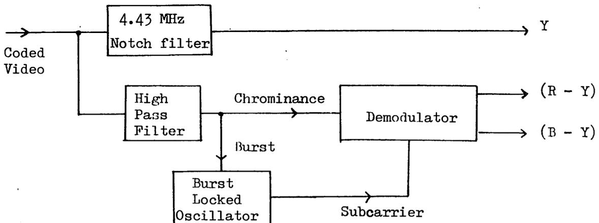
Fig. 4 : Simplified System Diagram of Decoder
