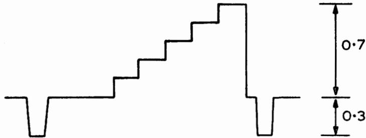
Figure 5.1: Five riser staircase waveform
