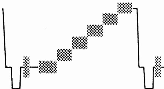
Figure 5.2: Staircase + subcarrier
