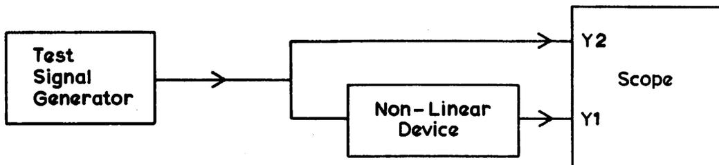
Figure 2: Comparison of signals using a differential 'scope
