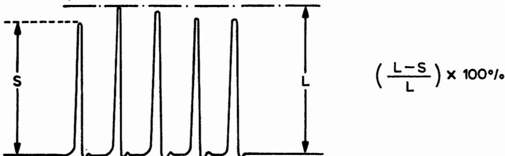
Figure 11: Calculation of Luminance non-linearity
