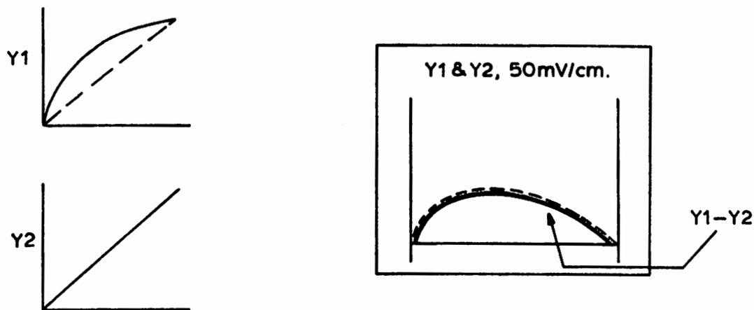
Figure 3: Gamma alignment using diff scope and graticule
