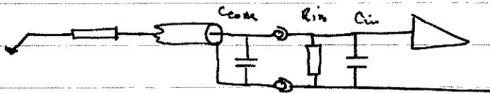
$$V_{\text{input to scope Amp}} = E_{\text{LF}} \times \frac{R_{\text{in}}}{R_{\text{probe}} + R_{\text{in}}}$$
