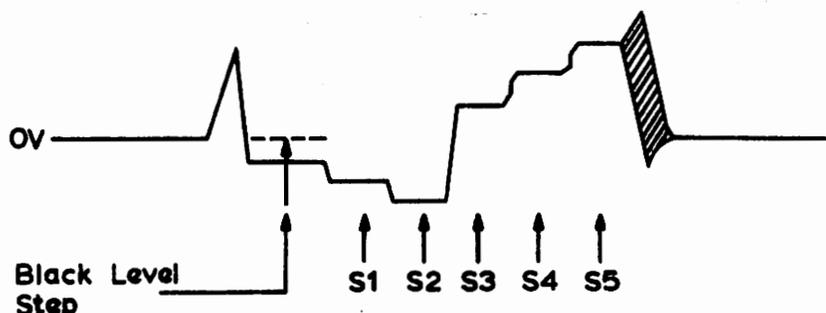
Figure 14: Typical diff. phase measurement display
