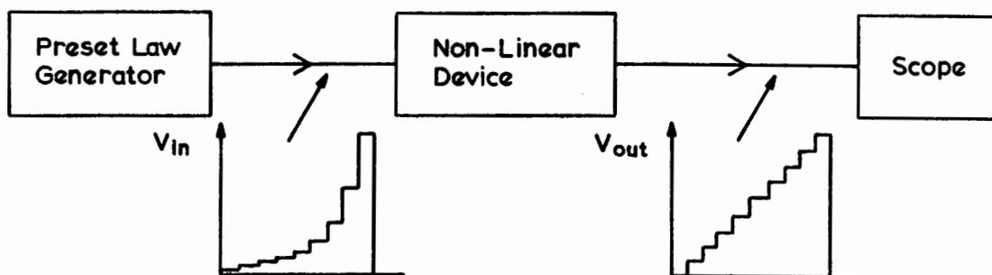
Figure 4: Pre-distorted Test Signal
