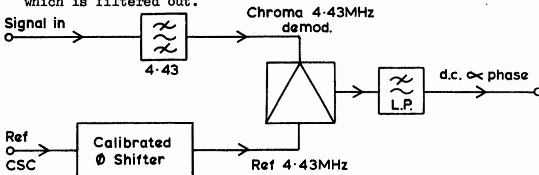
Figure 13: Simplified diagram of the phase detector
