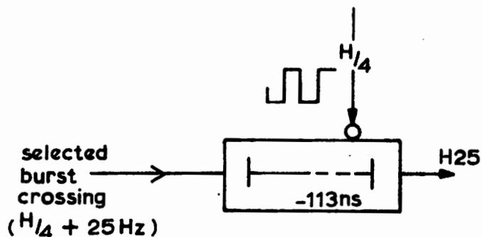
Fig. 4.3 Removal of 4-Line Sequence in Burst Crossing
