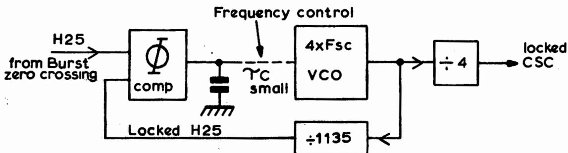
Fig. 4.4 Basic phase-locked Loop
