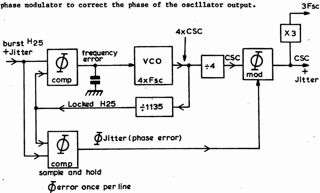
Fig. 4.5 P.L.L. with Output Phase Modulator
