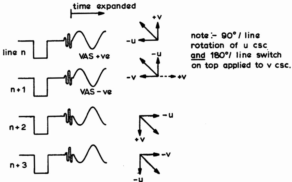
Fig. 4.1 Burst to Line Sync
