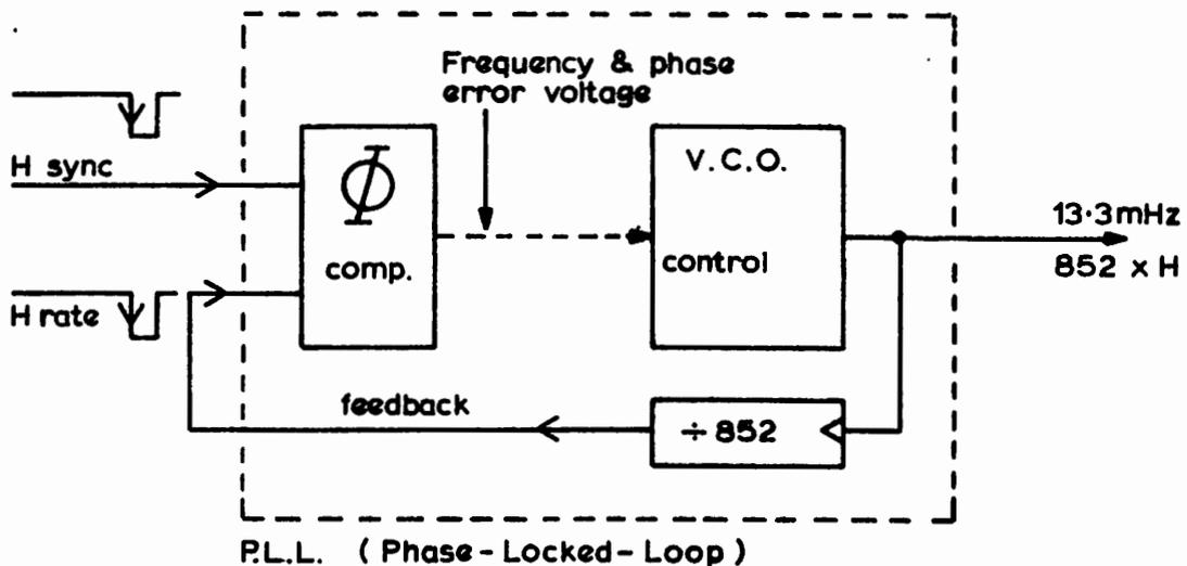
Fig. 1.1 Line-locked clock frequency
