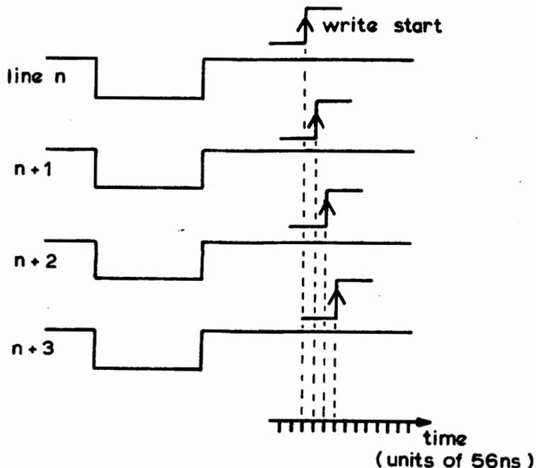
Fig. 2.2 'Write start' relative to line sync
