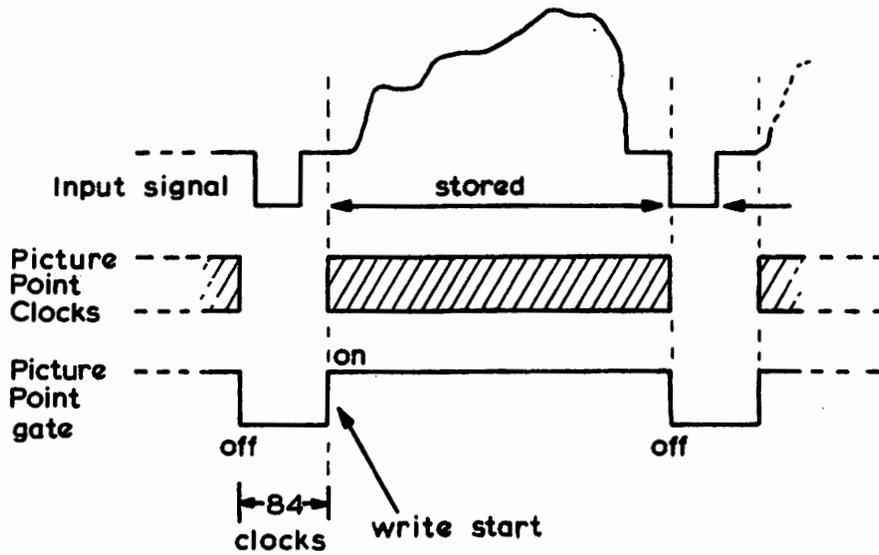
Fig. 2.1 Picture Point Clocks and Picture Point Gate
