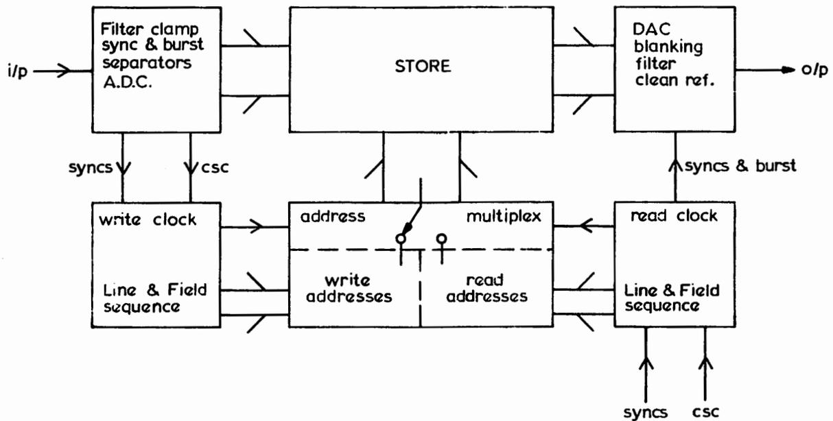
Fig. 0.1 Simple Store block diagram
