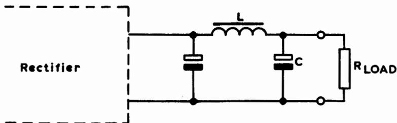
Fig. 6 : 'Capacitor input' filter
