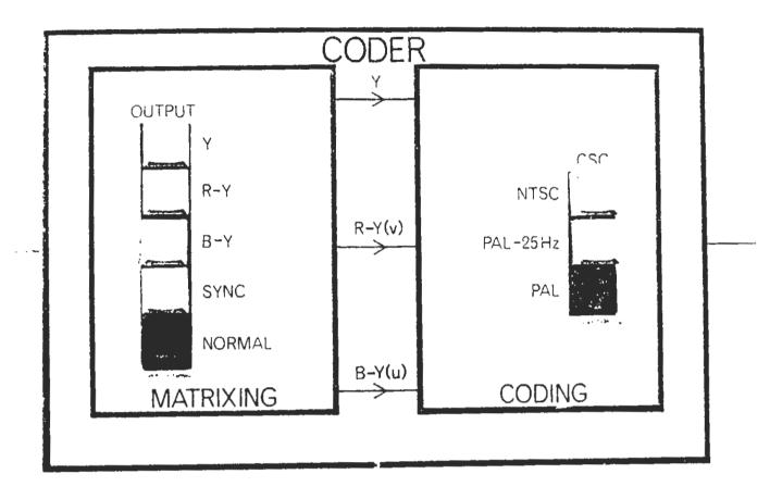
The Red, Green and Blue outputs of the Signal Source are fed via switches to the CODER. In the Coder these three signals are matrixed to provide separate luminance (Y) and colour difference signals, (R - Y) and (B - Y). Any one of these three may be used or the NORMAL operation adds the modulated colour differences signals to the luminance. The frequency of the subcarrier used in the modulators can be switched on the right hand (CODING) section of the Coder.
