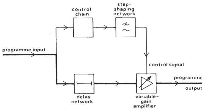
Fig. 7 Input-controlled limiter with step-shaping and delay networks.
