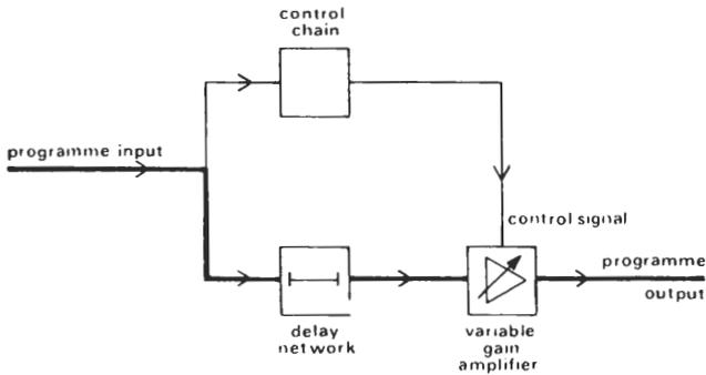
Fig. 6 Input-controlled limiter with delay network.
