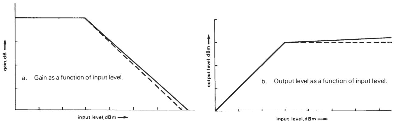
Fig. 2 Typical steady-state characteristics of simple limiter.
