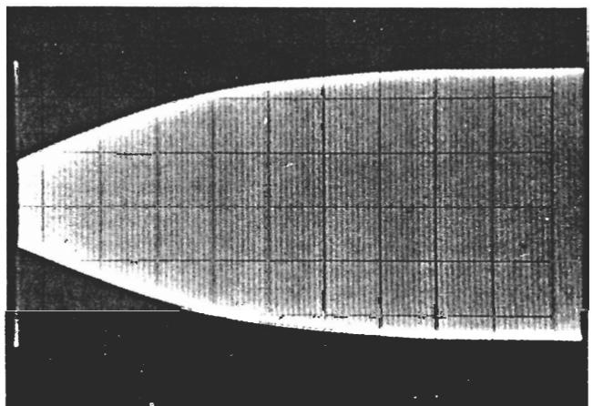
Fig. 3 Typical dynamic characteristics of simple limiter.
