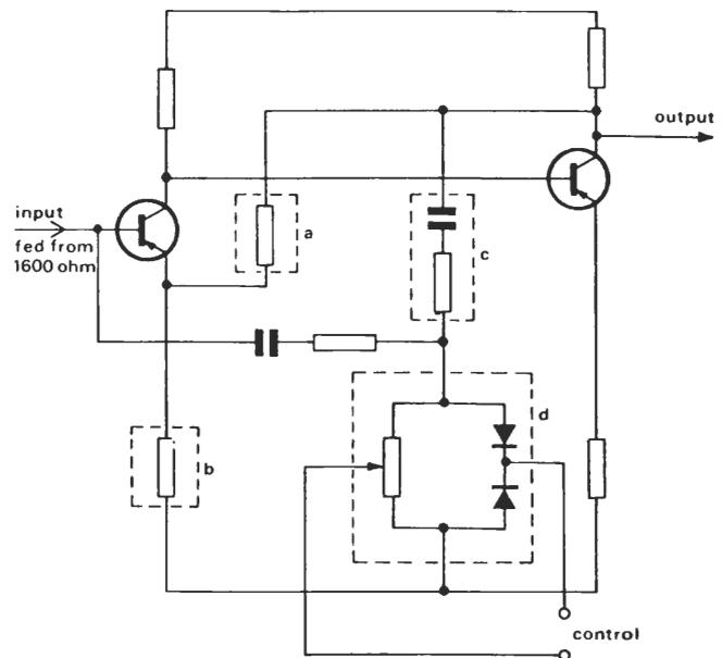
Fig. 5 AM6/3 variable-gain amplifier.
