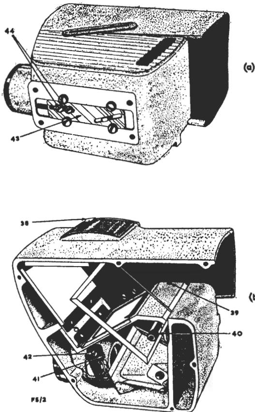
**Fig. 4.1. Two views of Auto-parallax Viewfinder, showing Adjustments**
