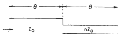
Fig. 29. Compound Short-circuited Line comprising two Quarter-wave Sections of different Z_0 in Series
