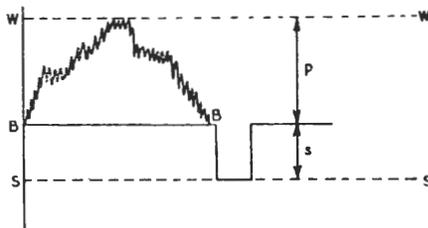
Fig. 5. Composite Waveform, showing  $p/s$  ratio.
