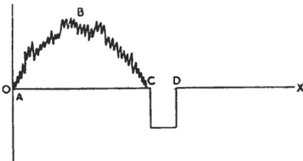
Fig. 4. Composite Waveform, Vision and Synchronising Signals
