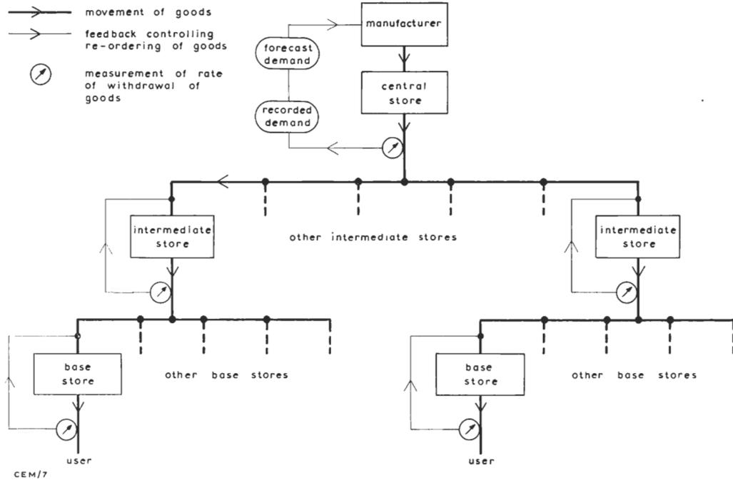
Fig. 2.1 Simplified illustration of the CEMAST valve-stores system
