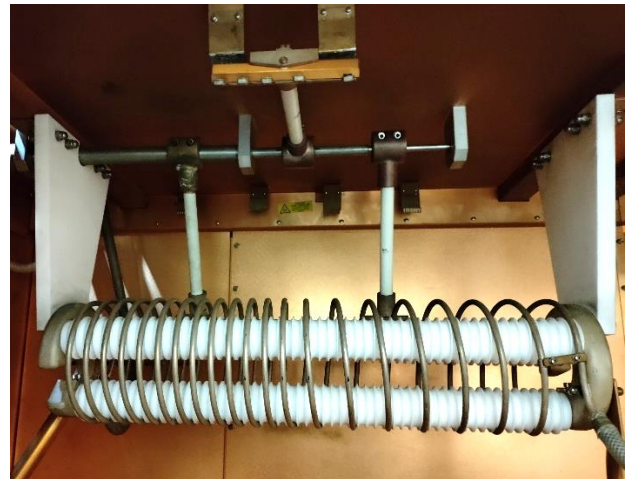
Figure 7. L305 part of the final RFC. This is water-cooled
