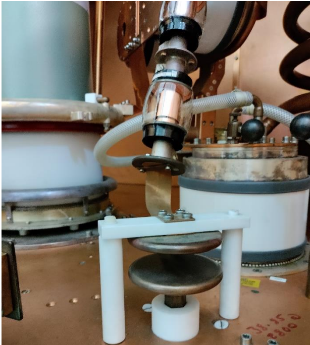
Figure 11. Motorised C314 neutralising capacitor and fixed series pair of C313 comprising 2 x 50 pF 55 kV vacuum capacitors
