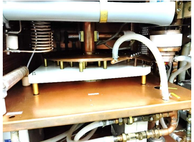
Figure 4. Control grid input tuning L301 "Pancake" coil (horizontal roller coaster, with water cooled tap and coil).
