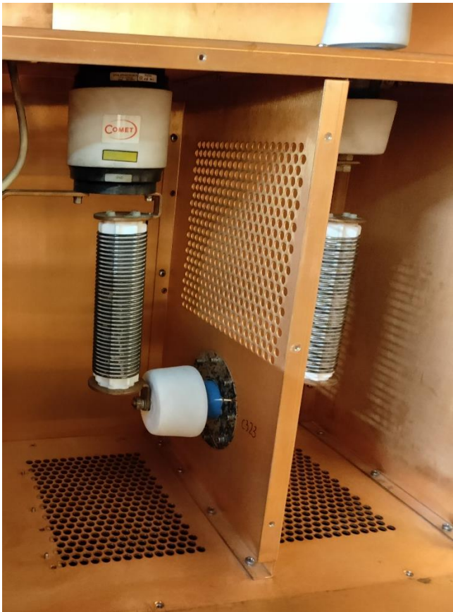
Figure 6. L307 and L306, part of the anode RFC, with the decoupling capacitors C324, C323 and C322
