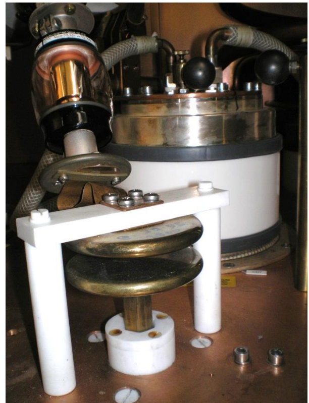
Figure 4. RIZ 250 kW sender showing motorised neutralising capacitor etc
