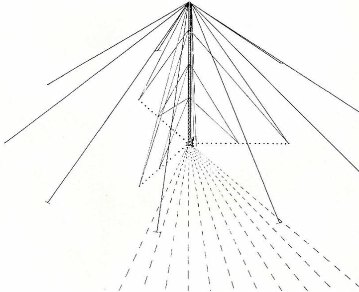
Figure 3. General arrangement of the R5071 antenna
