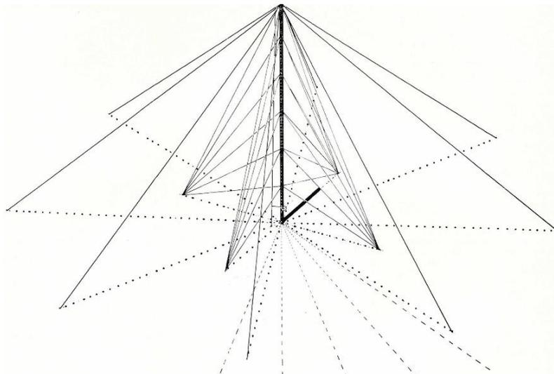
Figure 4. General arrangement of the R5075 antenna
