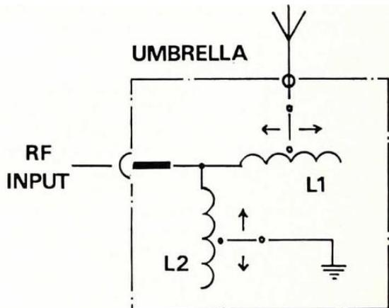
**Figure 5. Circuit diagram of the ATU for the R5075 antenna**
