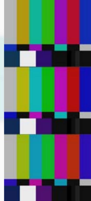
Effect of positive and negative phase errors on NTSC colour bars (correct at centre)
