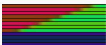
Here is a Simple PAL (PAL-S) display fed with a signal containing a large phase error. The error appears as different hues on adjacent pairs of lines, known as 'Hanover' or 'Venetian' blinds. With a PAL-D decoder employing a
