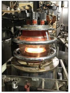
A BY1144L triode valve in the LH modulator position in a MWT BD272 transmitter (Neale Bateman)
