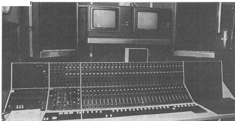
The 30-channel/ Glen Sound mixing desk, LS 3/7 monitor speakers, and monitor-receivers.
