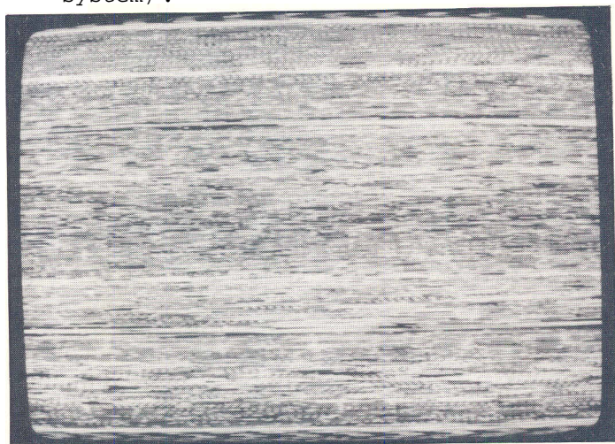
A picture scrambled by active line rotation a possible system for future subscription services (see page 3).
