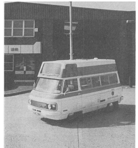
A radio-link vehicle, with its mast extended, outside the new Radio OB base at Acton
