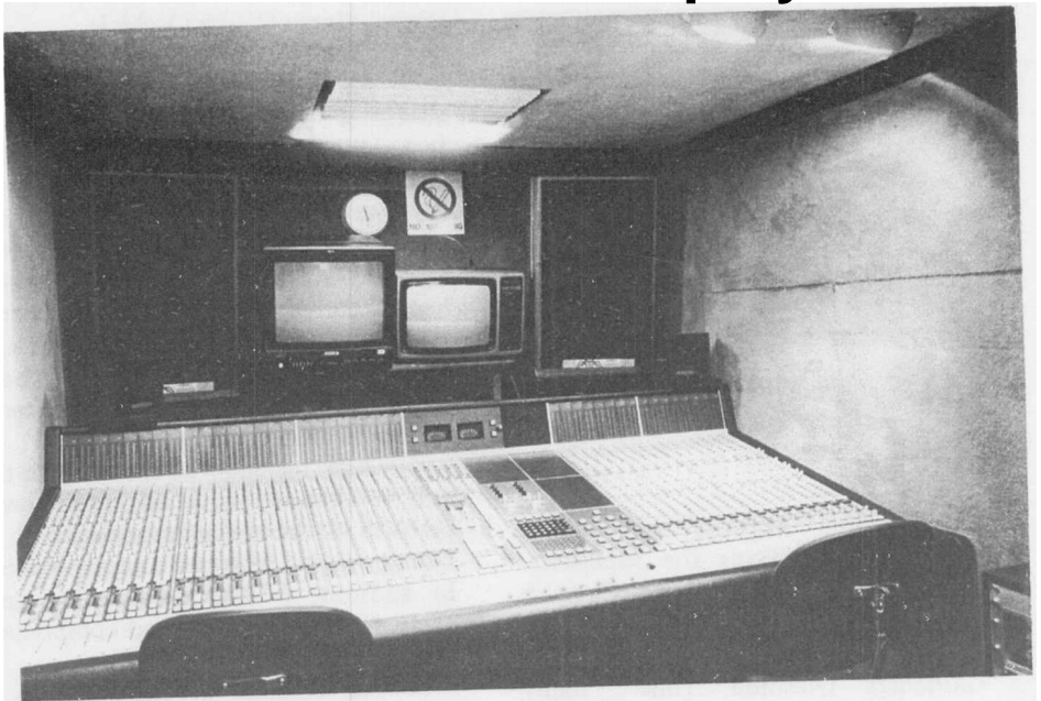
The Solid State Logic (SSL) computer-assisted control desk inside a Type A stereo control vehicle
