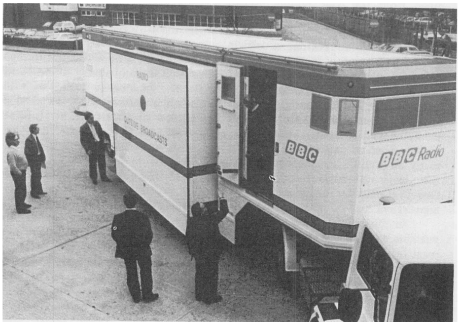
OB staff inspect the new expanding side digital stereo control vehicle
