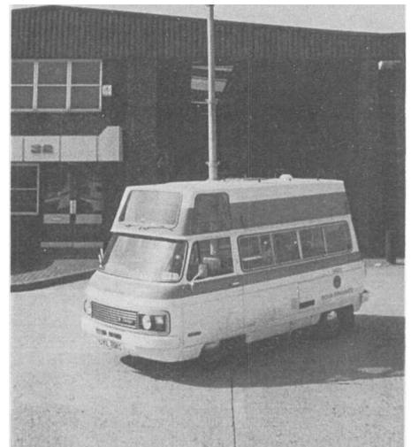
A radio-link vehicle, with its mast extended, outside the new Radio OB base at Acton
