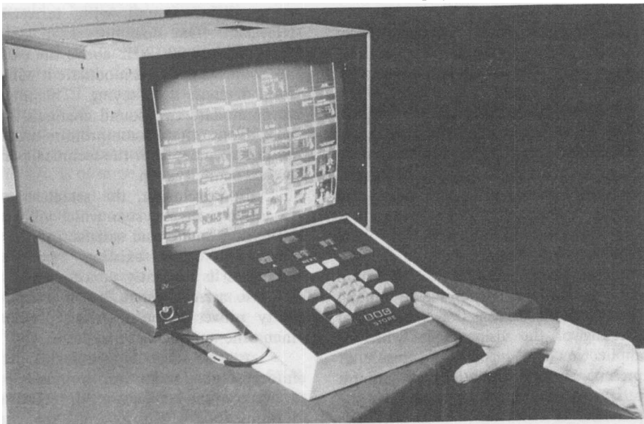
View of stills store controller.
